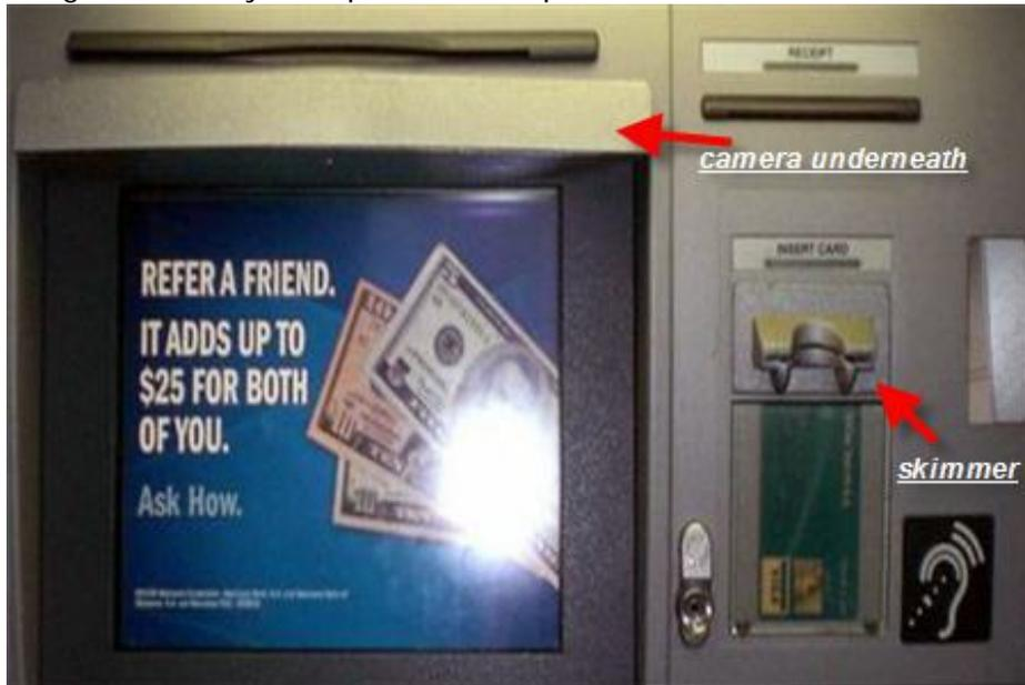
It is important to keep in mind that this attack is not trivial from an engineering standpoint. The shim needs to be extremely thin and flexible. In fact it must be less than 0.1mm in most cases to fit in the space allocated in the card reader and not obstruct credit cards from being inserted seamlessly. The EMV 4.2 standard [1] that regulates the dimensions of the card slot calls for the following specifications according to section 5.2.1.1 on Module Height:
